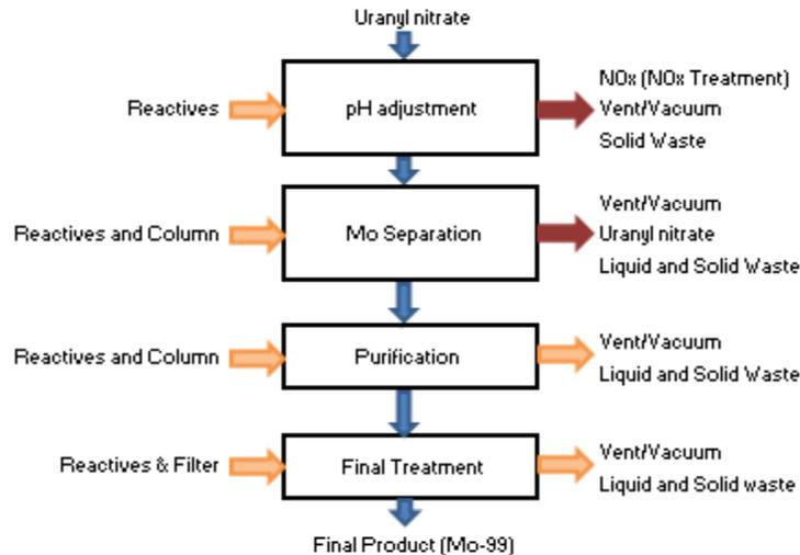
Figure 5: Block diagram of the processes in the shielded cell
