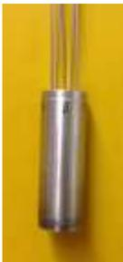
**Figure 8.** Micro-SHINE Phase II solution capsule.
