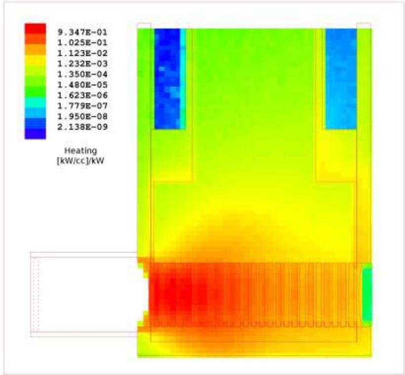
**Figure 2.** Power density distribution [kW/cm<sup>3</sup>] per kW of beam power for a 35 MeV beam and natural molybdenum disks. Simulated with MCNPX.
