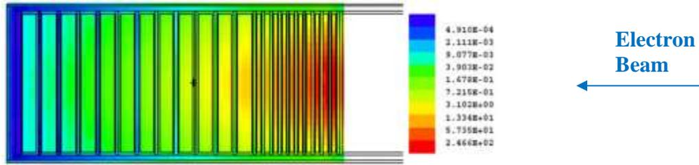
**Figure 7.** Energy deposition (watts/cm<sup>3</sup>/kW) in the depleted uranium photo-neutron converter, for the irradiation conditions given in the text
