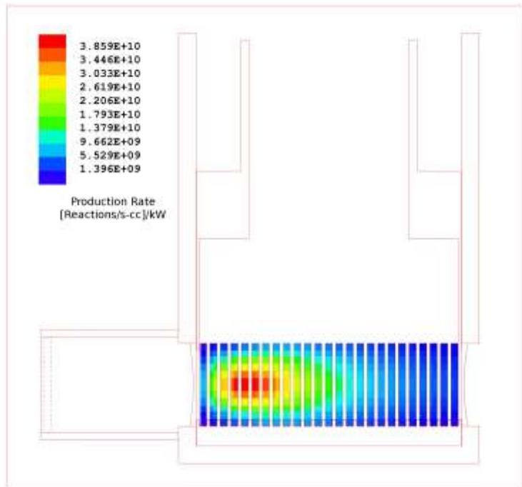
**Figure 3.** Mo-99 production profile [reactions/cm<sup>3</sup>-sec per kW] for a 35 MeV beam and natural molybdenum disks. Simulated with MCNPX
