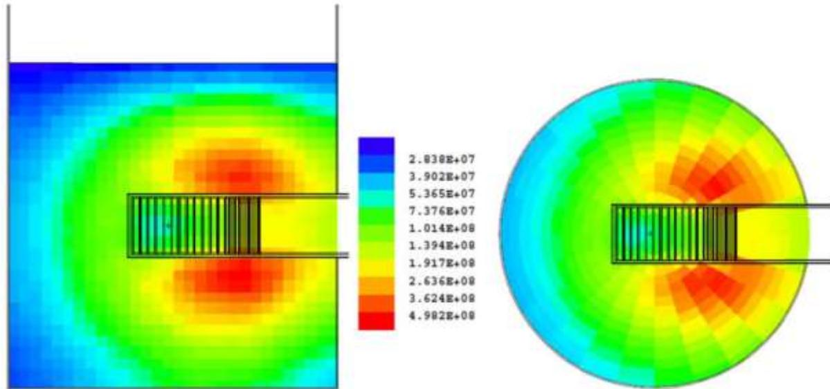
**Figure 9.** Fission rates (# fissions/cm<sup>3</sup>/kW) in the uranyl nitrate solution, for the irradiation conditions given in the text. Left - side view. Right - top view.
