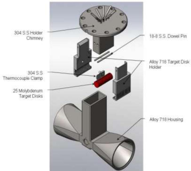
**Figure 1.** Helium cooled Mo-99 production target assembly for NorthStar experiments. Designed and implemented by Los Alamos National Laboratory
