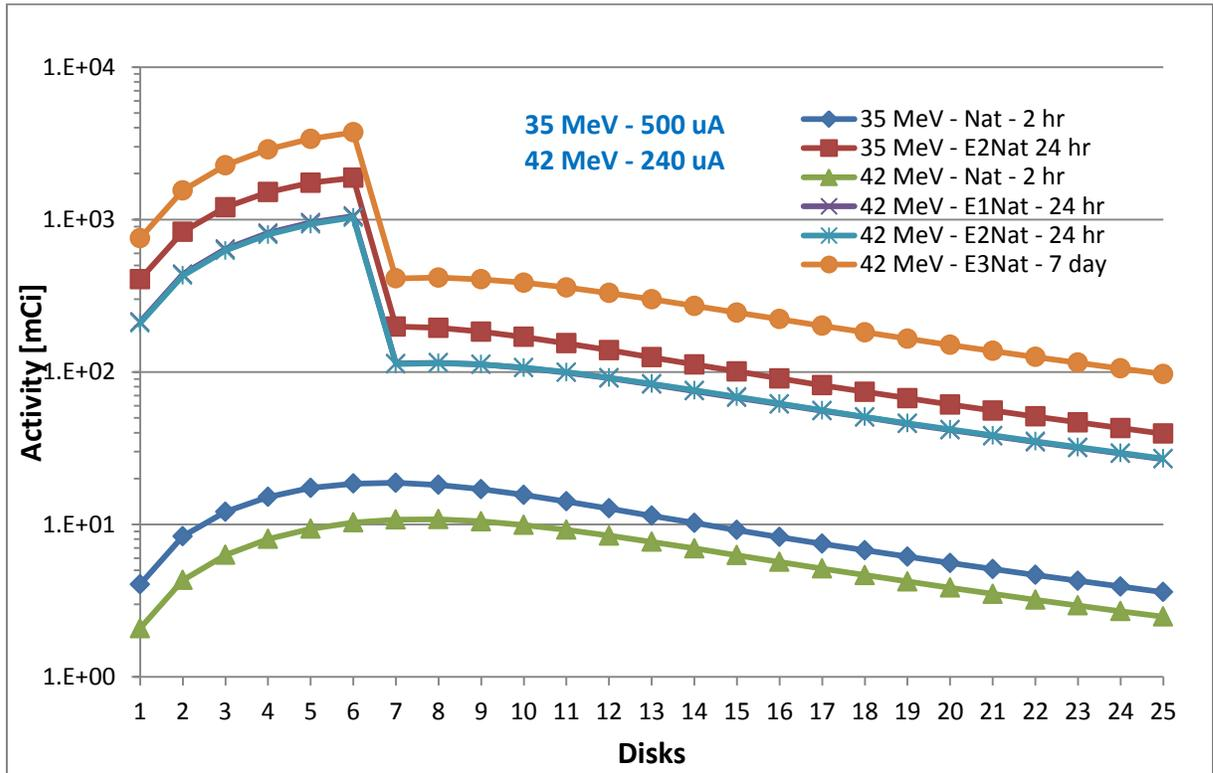
**Figure 4.** Disk by disk end of bombardment Mo-99 activities [Ci] for different target configurations and beam energies. Simulated with MCNPX
