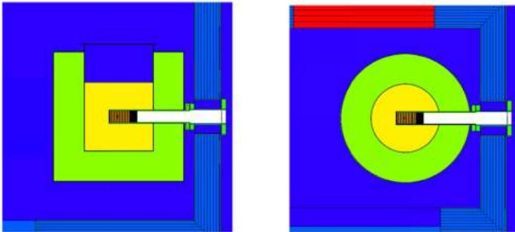
**Figure 8.** (left) Side view of MCNPX model used for DU target and uranyl nitrate solution calculations. The beam is incident from the right. (right) Top view of the MCNPX model through the beamline. The beam is incident from the right
