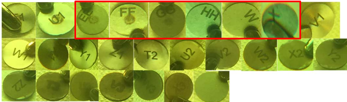
Figure 2. Photographs of 26 disks used in 4 th irradiation (see Table 1). Highlighted disks are ^{100}Mo enriched disks; the last disk on the bottom right is ^{98}Mo enriched disk
