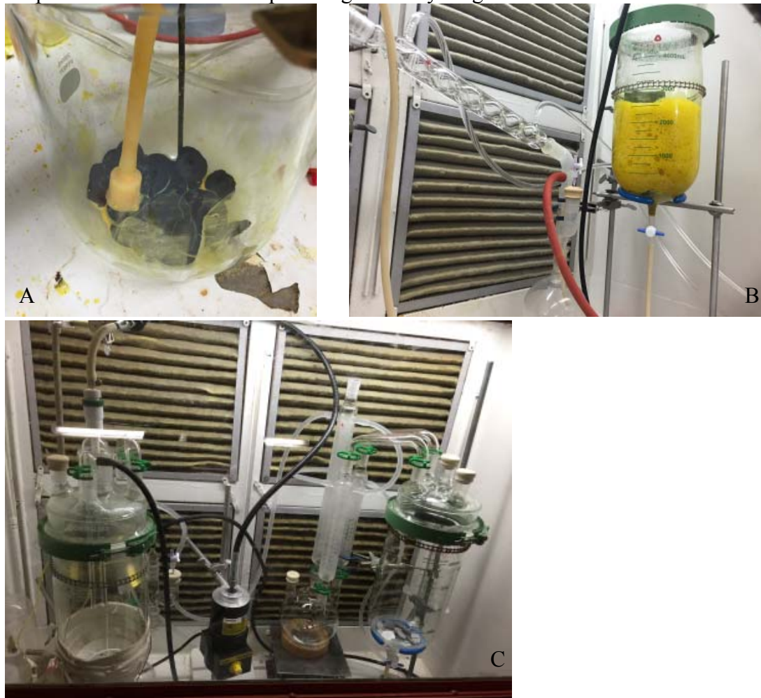
Figure 6. Setup used for dissolution of 75-300g of sintered Mo disks using 30-50% hydrogen peroxide
