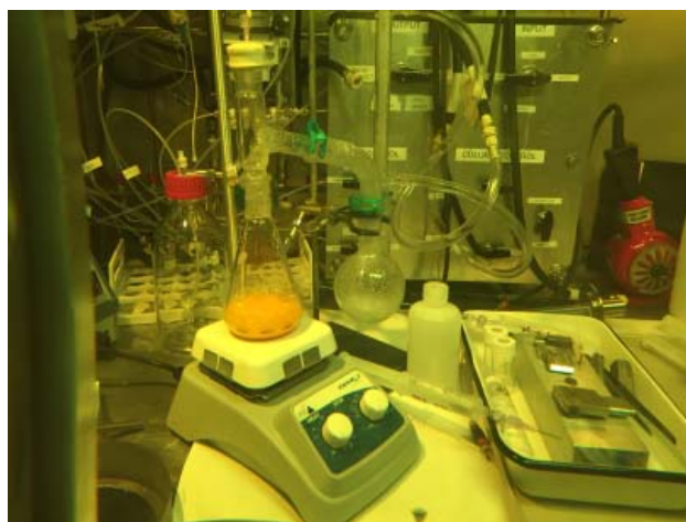
Figure 4. Dissolution apparatus used for dissolution of six ^{100}\text{Mo} enriched disks
