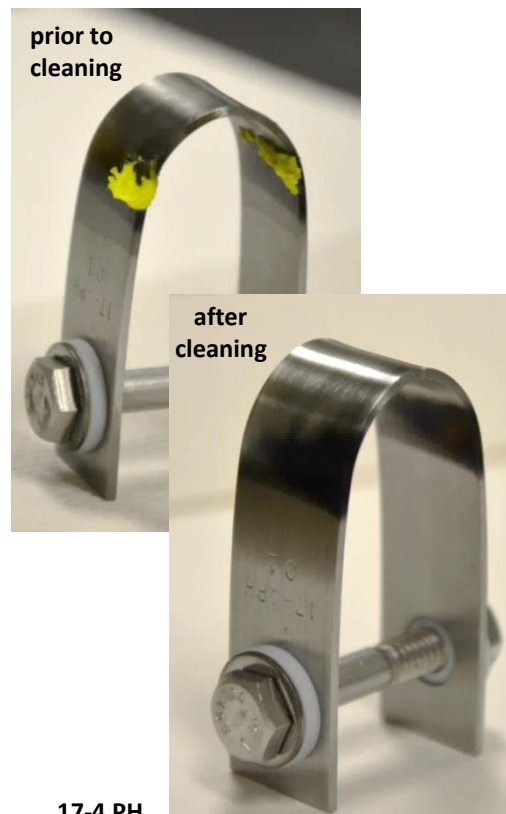
17-4 PH 140 g dU/L + 0.1 M excess \text{H}_2\text{SO}_4 after 10 days at 80-81°C
