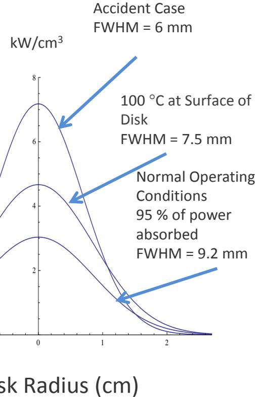
The volumetric heat generation rates presented here assume an electron beam power of 20 kW
