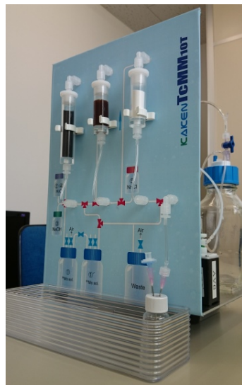
10TBq type, AC-IER-AL columns
