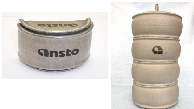
Figure 3-5 Hot-isostatically pressed dumbbell-type cans used for Pu-doping work. The can uncut on the left contained \sim 370\text{ g} of zirconolite-rich Synroc containing \sim 50\text{ g} of \text{PuO}_2 and 18 wt% Gd, Sm and Hf neutron absorbers. The can is \sim 6\text{ cm} diameter by 4\text{ cm} high. The can on the right is a non-radioactive 5 kg scale up, \sim 9\text{ cm} diameter by 18\text{ cm} high. The final size can be tailored by adjusting the starting geometry of the cans.
