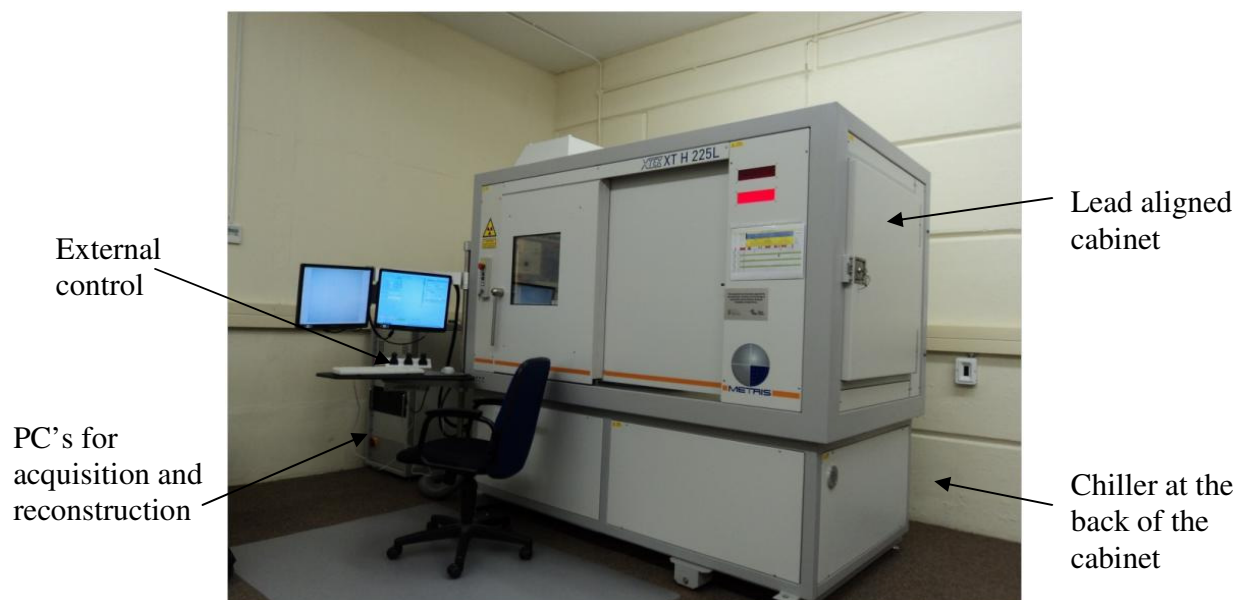
Figure A-1 Micro-focus X-ray machine at the MIXRAD facility
