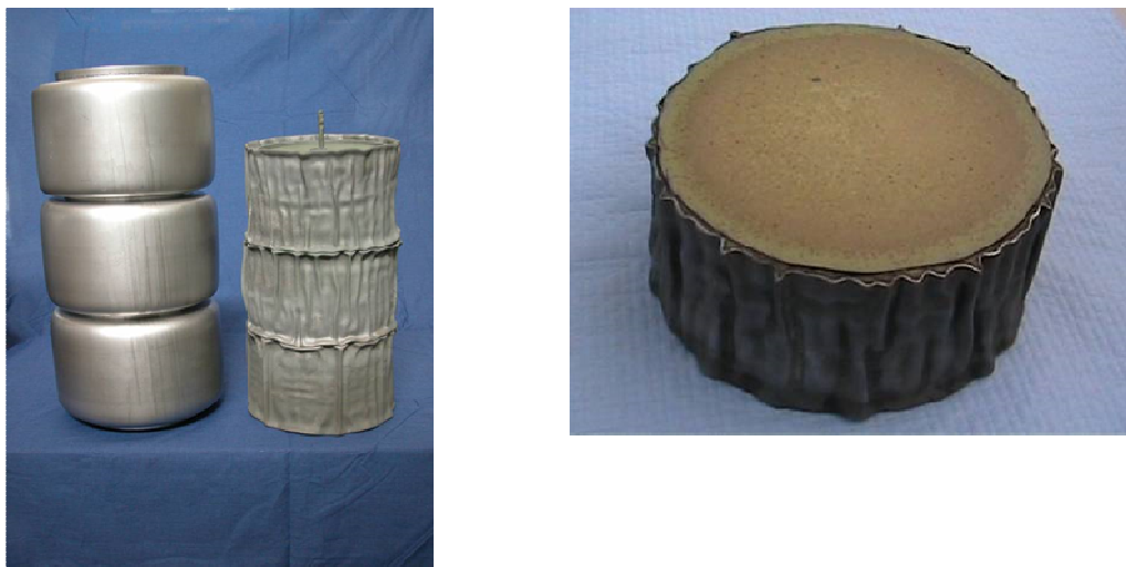
Figure 6-11 First non-optimized 30 kg scale HIP demonstration of the Zr-calcine (80 wt% waste loading) simulant. HIP can before and after (left) and cut section (right).
