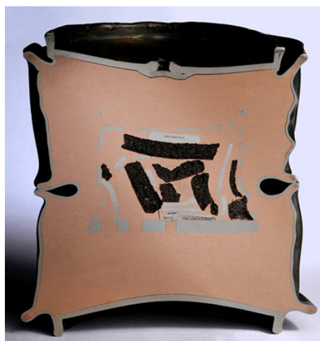
Figure 6-10 Sectioned HIPed copper metal encapsulation waste form containing uranium-aluminium alloy, cermets, steel and graphite. Note the U-metal (Mo-99) target emplaced in the sample.
