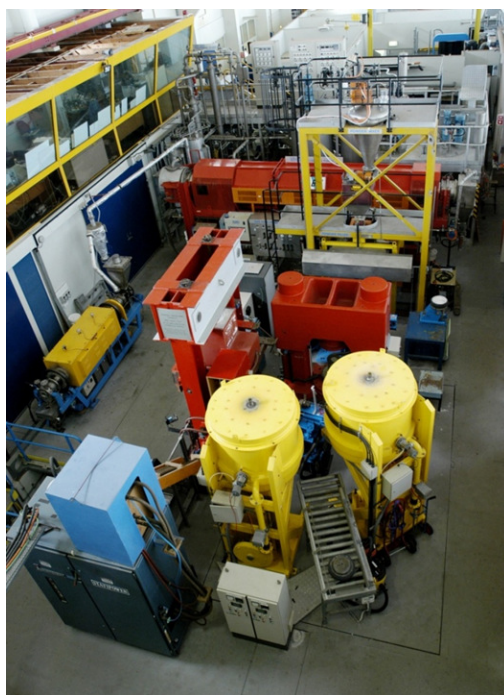
Figure 6-1 The Synroc Demonstration Plant, designed to produce 10 kg/hr of Synroc. At the top are the mixing tanks for the simulated waste and precursor; this was fed into a rotary calciner (red). In the foreground are the preheating and cool-down furnaces (yellow). The plant also contained a cone blender into which Ti metal was blended with the product exiting the calciner, a filling station which filled the metal bellows, a prepress, robotic arms to move the cans, and an induction heated hot-press (Figure 6-2). On the left is a smaller rotary calciner (yellow and blue) for a dry-feed route.
