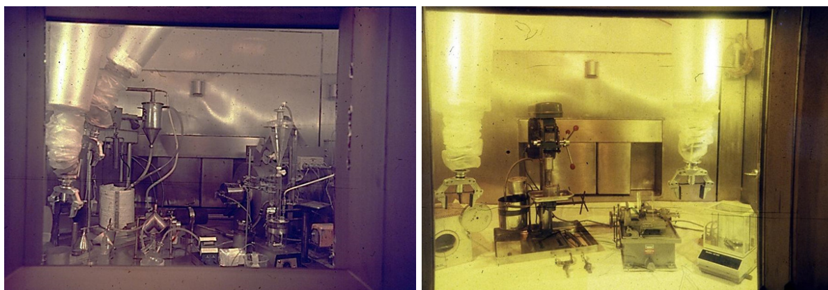
Figure 6-4 Two of the hot-cells used to produce Cs-137 and Sr-90-doped Synroc at ANSTO. The top cell was the processing cell; it contained a pot mixer dryer, a rotary calciner, a V-blender, hot-press and other ancillary equipment. The second cell was the test sample preparation cell with sample coring, cutting, weighing, density measurement and leach test apparatus.
