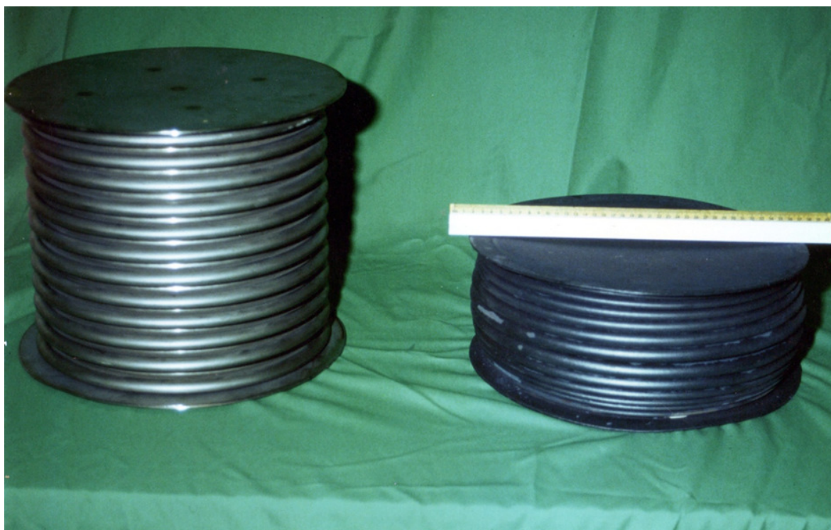
Figure 6-3 An early hot-uniaxial pressing bellows containing ~ 40 Kg of Synroc-C showing the bellows before (left) and after (right) hot pressing. The ruler is 40 cm long.
