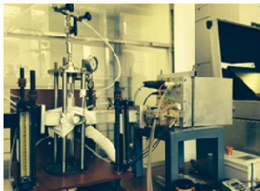
Figure 6-13 Use of microwave technology to apply SiC coatings onto substrates
