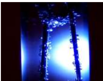
Figure 5. Bubble formation and Cherenkov radiation were seen in the mini-scale bubble experiments at the VDG (1.3 M \text{NaHSO}_4 solution, \text{pH} = 1.28 , beam current is 22\mu\text{A} ).
