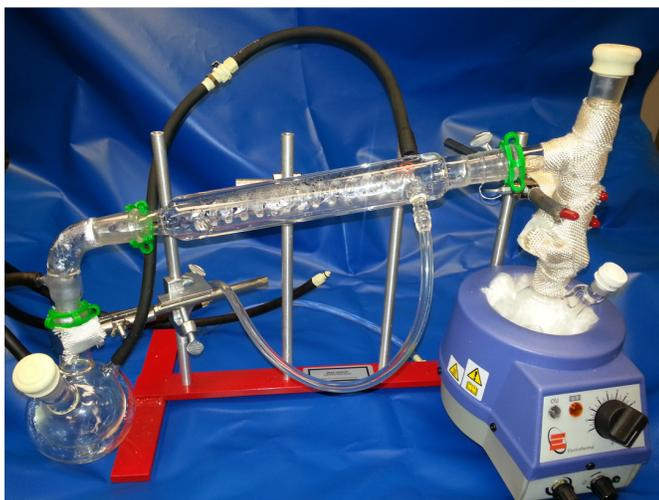
**Figure 5.** Evaporation apparatus: Collection flask (left) water cooled condenser (middle), insulating tape-wrapped adapter (right), evaporation vessel (right), heating/stirring mantle (right). Septa were used to allow for addition of solvents and removal of solution via needles and cannulas. Quick-connect valves were utilized for the water lines.
