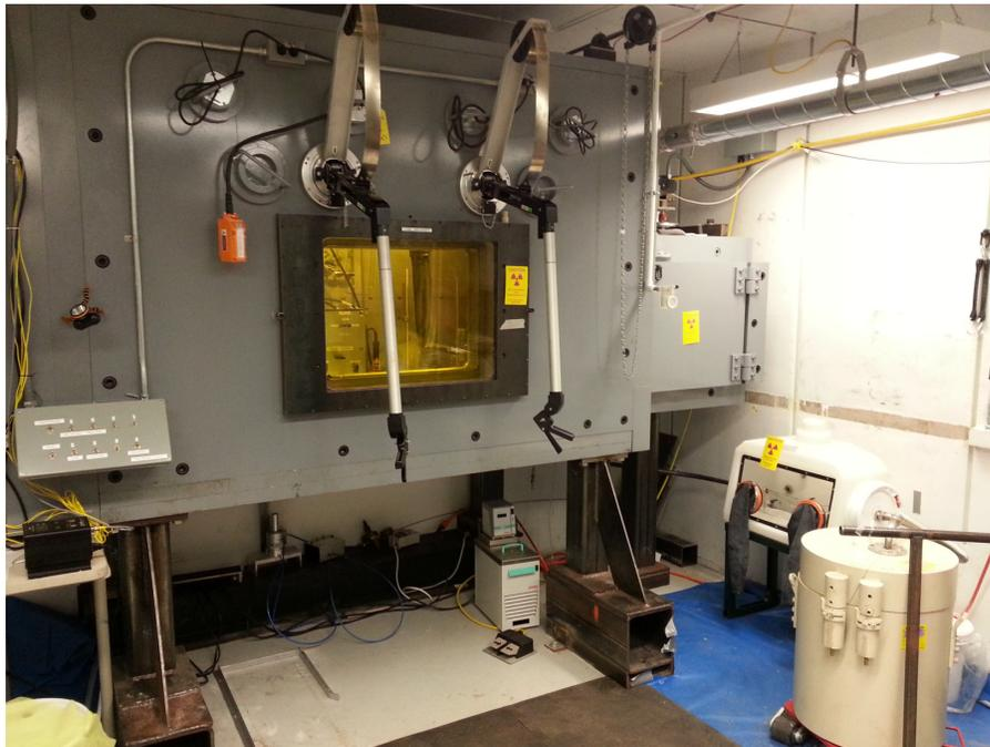
**Figure 2.** Image of Bigfoot hot cell used during concentration column, evaporation, and LEU-Modified Cintichem processing. The identical white intermediate transfer glove box and transfer cask are also shown.
