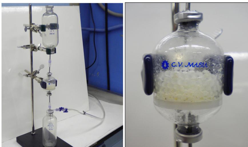
**Figure 8.** Image of Cintichem filtration step (left) and non-modified fritted vessel (right).
