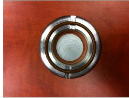
(left) TRIUMF-designed, GE PETtrace solid target capsule; (right) with mounted ^{100}\text{Mo} target Reference: P Schaffer, personal communication.
