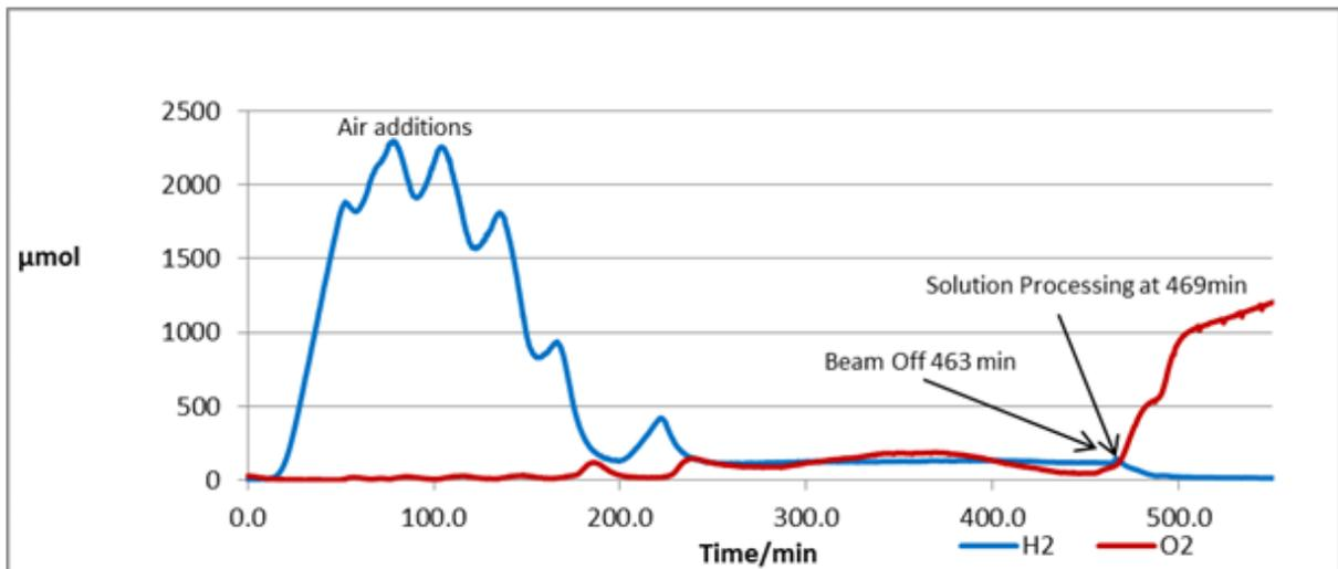
**Figure 4.** Hydrogen and oxygen generation rates during the second LEU uranyl sulfate irradiation.
