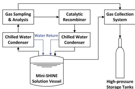
**Figure 1.** Block diagram of the mini-SHINE gas analysis and collection system.
