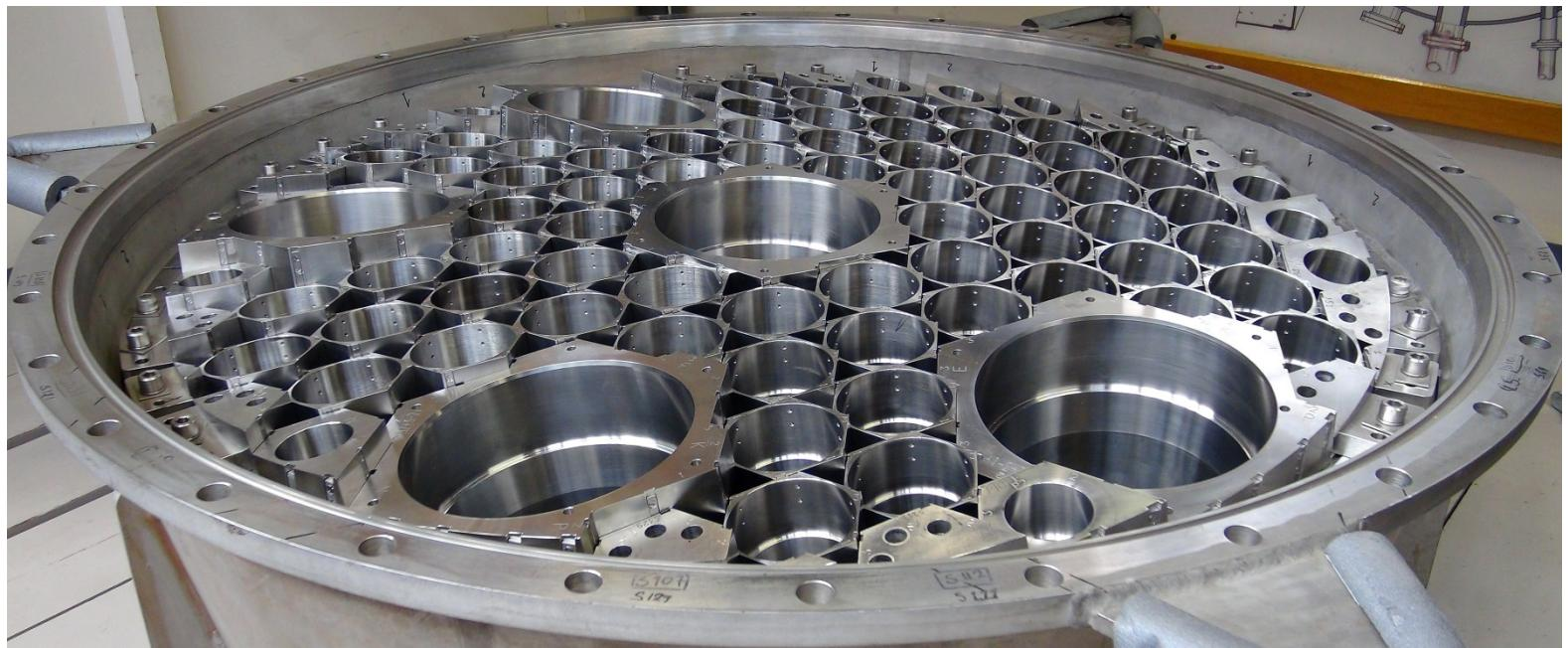
**The new beryllium matrix will be installed in BR2's pressure vessel begin of 2016 after the pressure vessel inspection programme scheduled in September – October 2015.**
