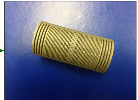
Notional 3D target design printed in stainless steel
