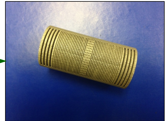
Notional 3D target design printed in stainless steel
