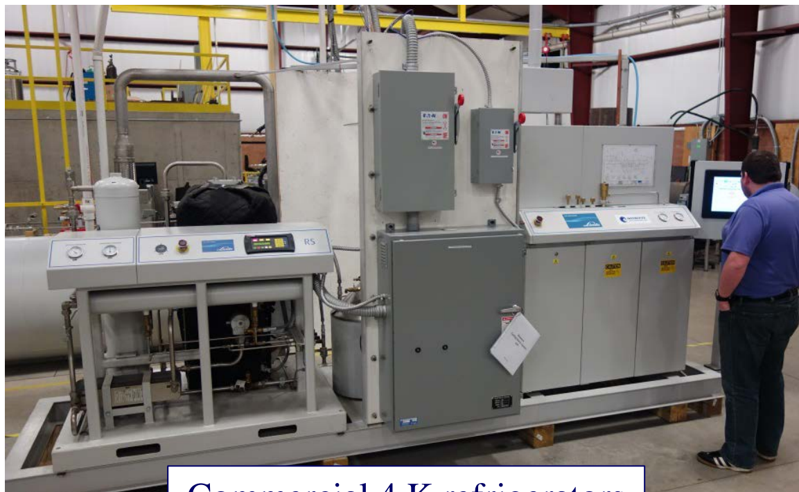
Commercial 4 K refrigerators (rugged piston-based systems, 100 W cryogenic capacity)
