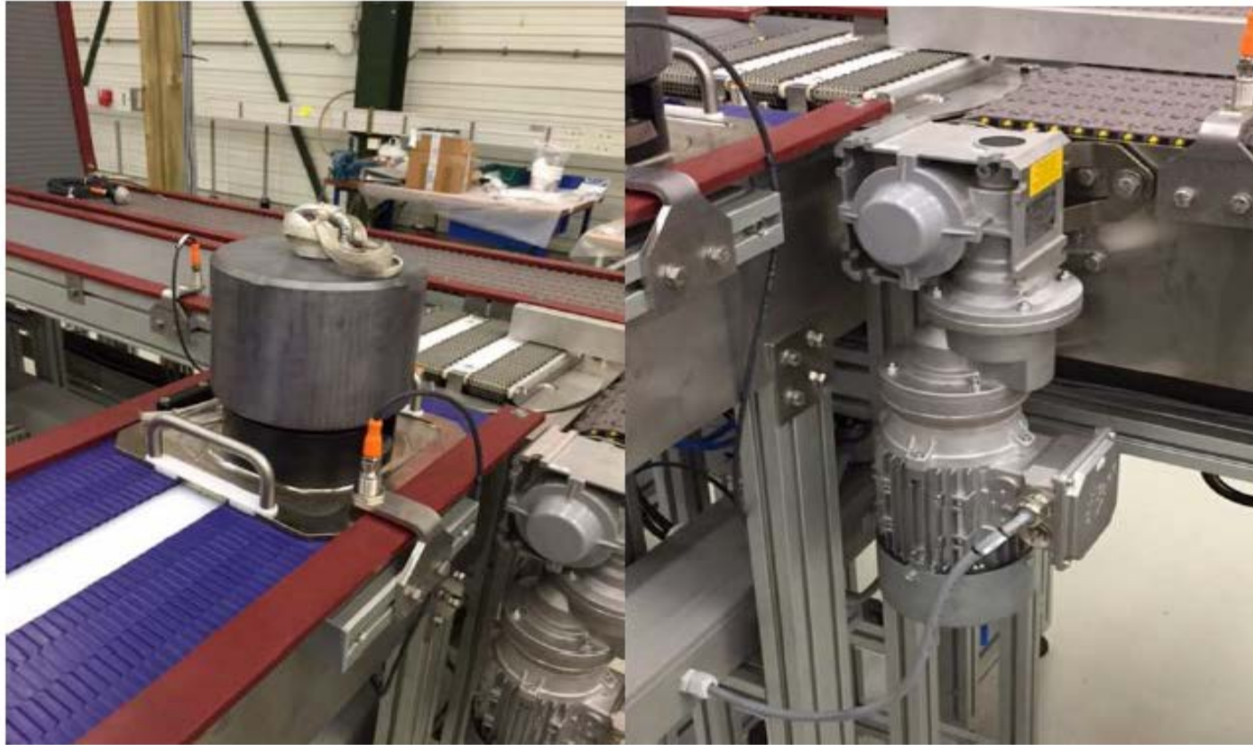
Conveyor belt details (simulated SV on left, drive motor on right)
