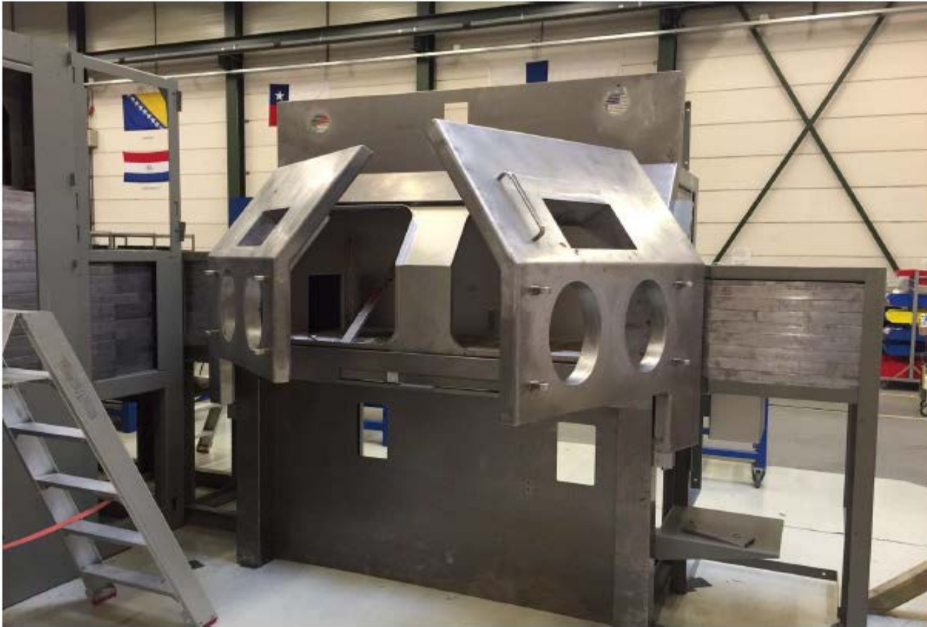
MURR2 – source vessel inspection glove box
