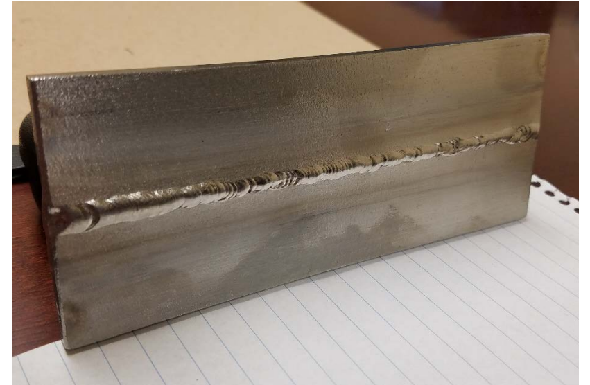
Burn through on the root side
